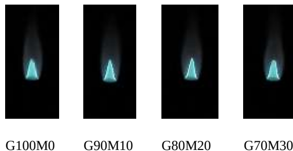
Figure 3. Flame with a fuel flow rate of 0.5 ml/minute
